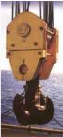
600 tonnes WLL Offshore Service Block. Quadruplex Hook
