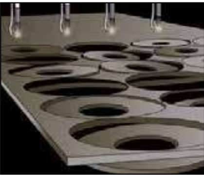
Each ForgeFab® sheave begins as driven, precision disc cut from proprietary chemistry alloy steel plate.
